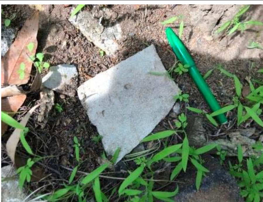
Image 6.10.1 View of example of potential asbestos containing materials on surface of site adjacent to eastern end of northern site boundary
